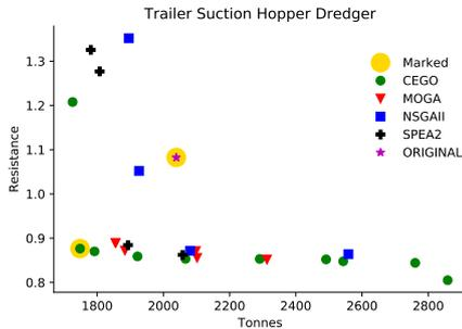
**Figure 5.3.1:** Original design and Pareto frontier obtained by CEGO, MOGA, NSGAI and SPEA2 on the dredger optimization problem.
