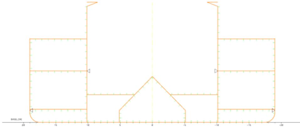
**Figure 3.2.3:** Schematic cross-section view of main frame scantlings.
