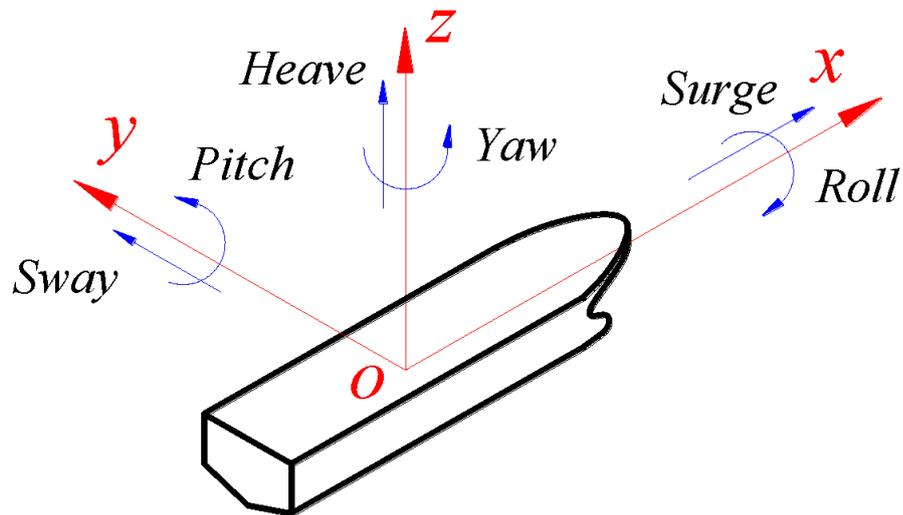
Figure 2.3.4: Roll, pitch, yaw, heave, sway, surge of a ship.
