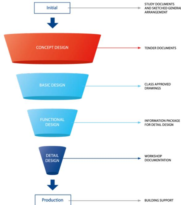
**Figure 3.1.1:** Four ship design stages: Concept-, basic-, functional- and detail design.
