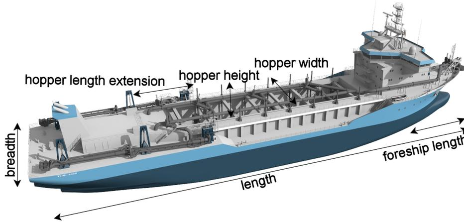
**Figure 3.2.1:** Trailer Suction Hopper Dredger designed by C-Job Naval Architects, with the design variables annotated.
