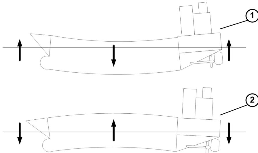
**Figure 2.3.2:** Ship hull is sagging in (1) and hogging in (2). Note that the bending is exaggerated.
