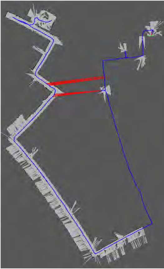
(a) The current map is visible with the detected loop closures in red.
