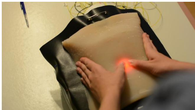
Figure 1: Participant is applying force on vertebra inside the prototype during user test.
