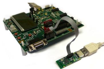
Figure 6: USB dongle connected to SmartRF board [7].
