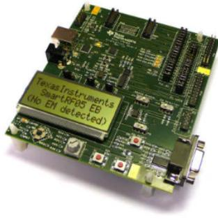
Figure 1: SmartRF05 evaluation board [7].
