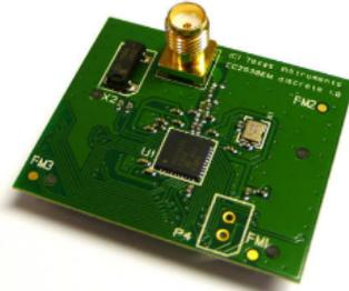
Figure 2: CC2530 evaluation module (without antenna) [7].
