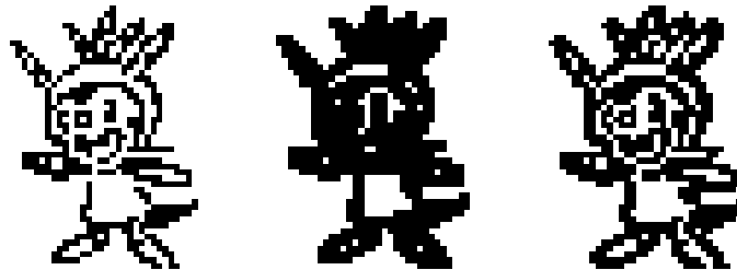
Figure 28: (a) Initial base puzzle ; (b) Binary erosion with a block 2 \times 2 kernel on the base puzzle ; (c) Modified erosion on the base puzzle
