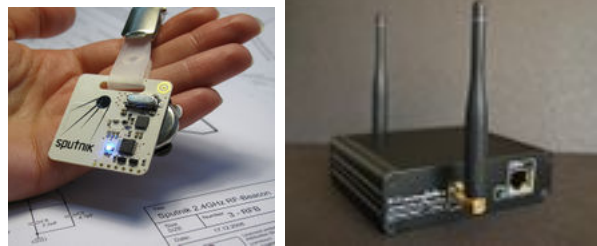
Figure 4: A tag for the OpenBeacon [19] and the OpenBeacon Reader.
