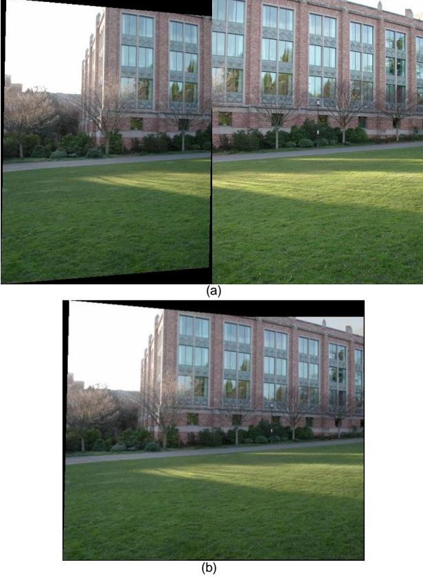
Fig. 6 (a) are the warped version of the two images, the image on the left is warped using geometric transformation according to the right image. (b) shows the two warped images stitched together.
