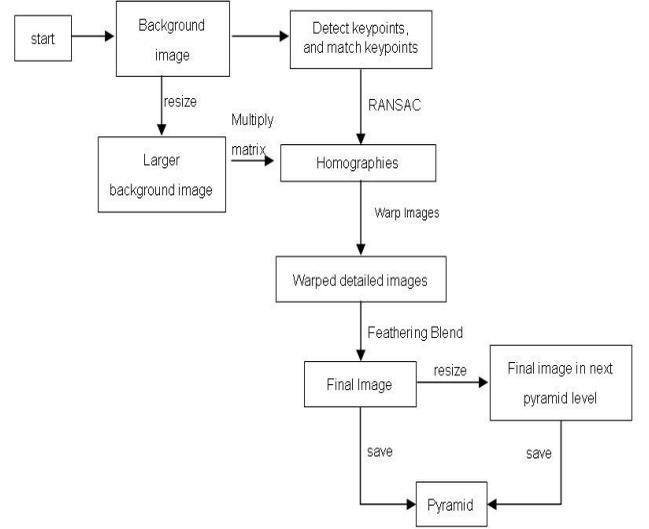
Fig. 12 The overall structure of the framework
