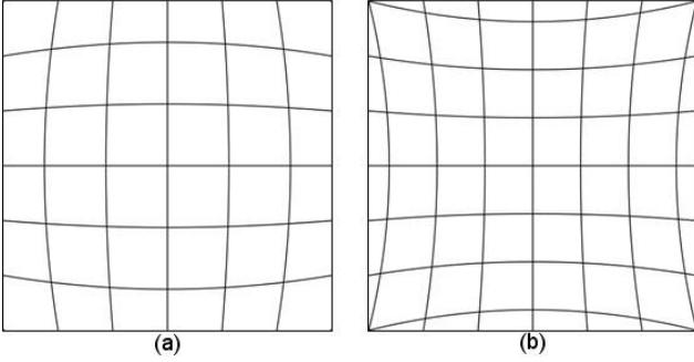
Fig. 2 Examples of radial distortion: (a) barrel and (b) pincushion.
