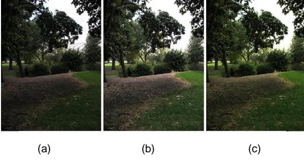
Fig. 4 The results of applying color correction: (a) is the original image, (b) shows the result of diagonal model, and (c) is gain compensation. Both (b) and (c) show the results of adjusting color of the right image according to the left image in Fig. 3.
