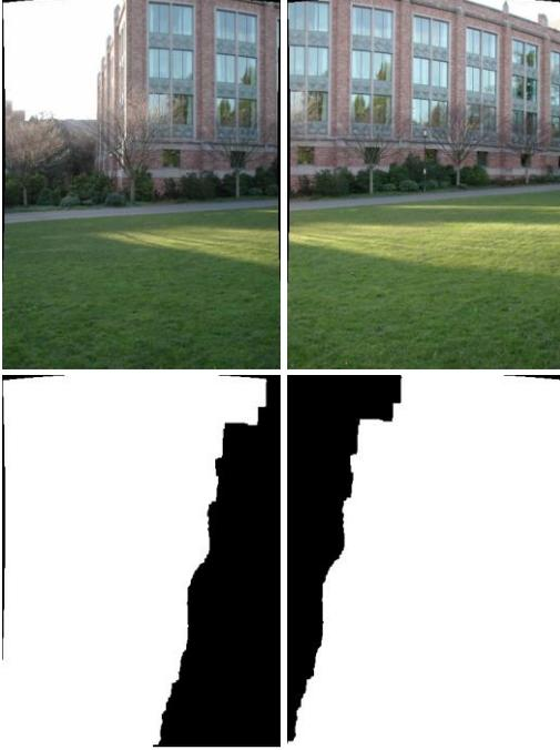
Fig. 9 The 2 images in the upper row are the 2 cylindrical warped images and the other 2 images are the masks, in which white part denotes the valid pixels and invalid pixels in black part.
