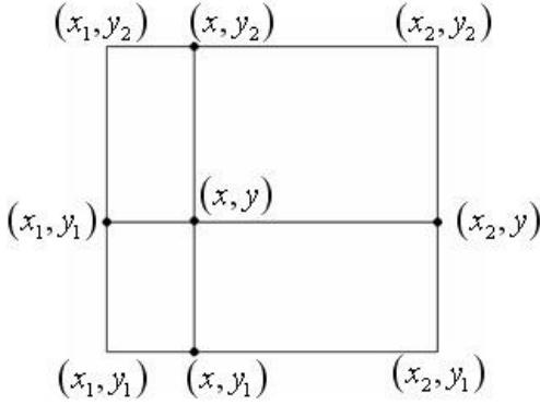
Fig. 5 Illustration of Bilinear Interpolation
