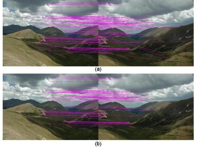
Fig. 1 (a) shows the preliminary keypoint matches, and (b) shows the inliers after applying RANSAC, where the mis-matches are pruned out.
