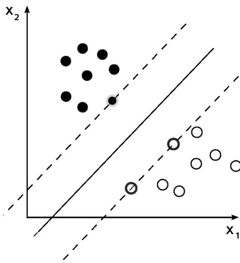
FIGURE 3.3.1. Maximal margin hyperplane for a trained SVM separating samples from two classes in the  $x_1$ - $x_2$ -feature space
