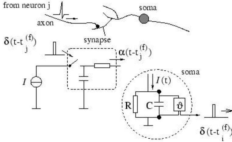
Figure 3.5: Schematic on which the leaky integrate and fire model is based. The main circuit is inside the dashed circle. The RC circuit is charged by a current  $I(t)$ . When the voltage  $u(t)$  reaches the threshold  $\vartheta$ , an output pulse is emitted. The circuit inside the square circuit models a synaptic connection.
