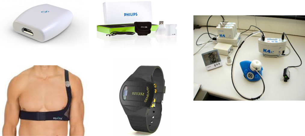
Figure 3.1: The devices used in GOTOv study. Active8 and Equivital (right), Philips DirectLife and GENEActive (middle), COSMED K4b2 (left).
