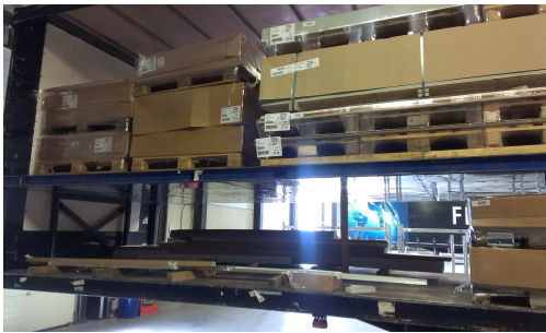
(a) Front Part of the Trailer. The front part of the trailer showing the raised area (bridge) present in some of the trailers under investigation.
