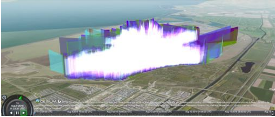
Figure 3.15: KML imported as KmlDataSource in Cesium. Note the white glow, probably caused by the partial transparency of the line stretches that is handled peculiarly by Cesium (i.e. the colours of the semi-transparent layers are added to form a white colour, instead of the semi-transparent layers only letting part of the ‘light’ pass through as would be natural).
