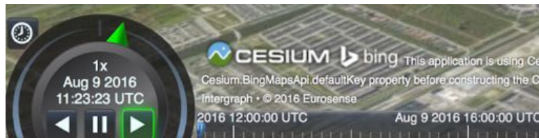
Figure 3.16: A detailed look at the Cesium time controller. Note the green arrow that designates the speed at which time moves (it can be dragged around the circle to increase or decrease the speed of time) and the blue marker at the start of the time line denoting the current time frame. The date and time of the current time frame are also displayed in the centre of the circle. The button at the top left, displaying a clock icon, resets the time frame to the current, real, time.
