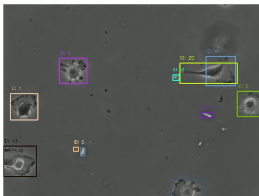
Figure 16: Case where two boxes find the same cell, but they are too different to have a large enough IoU to be considered boxes around the same cell, and one is not completely contained within another
