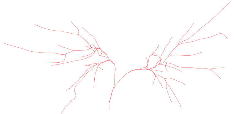
(b) The calculated one voxel thick centerline model without the original mesh.
