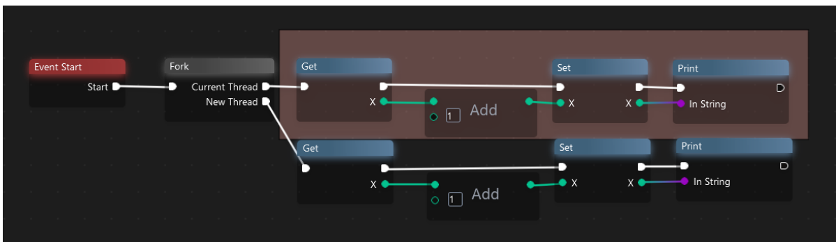
Figure 13: Wrong mutex usage. New thread is not locked out of executing.
