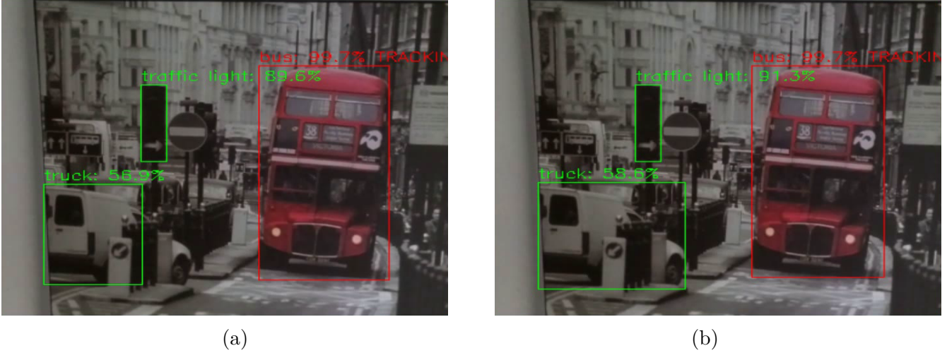
Figure 6.4: Bounding box inconsistency example. Large size change from frame (a) to (b) on the truck object
