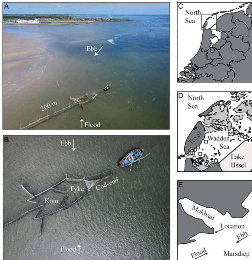
Figure 8: The NIOZ kom-fyke in the Dutch Wadden Sea. (A), (B): Aerial photograph showing the location and the design of the kom-fyke. (C), (D), (E): The map showing the location of NIOZ kom-fyke (Dark grey = land. Light grey = intertidal areas. White = water.) (Picture by Van Walraven et al. [20])
