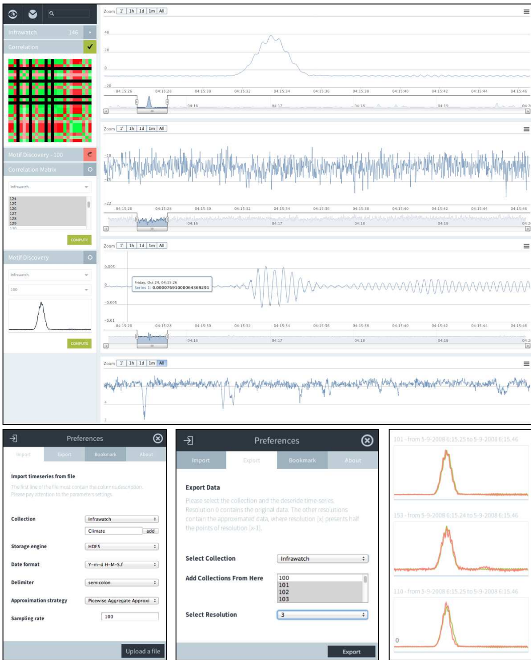
Figure 3.1: VizTool screenshot. a. The right side depicts the massive time series visualization structure. The left menu allows the usage of several data-mining components to the displayed time series. b. Data import form detail. c. Data export form detail. d. Detail of motifs discovered by using the tool.
