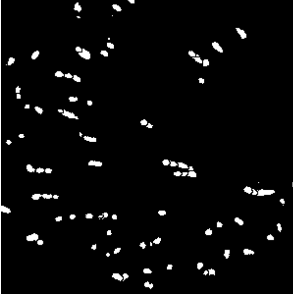
Figure 20: The binary mask from applying local Otsu segmentation combined with watershed algorithm on image in figure 18-A.
